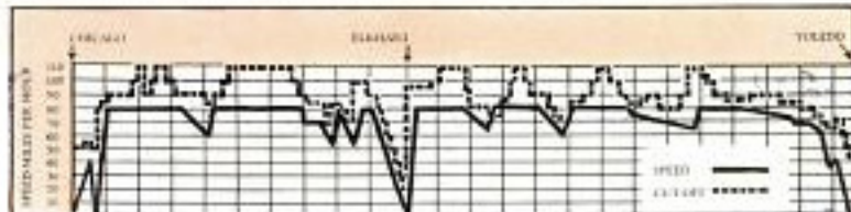
Top, the "Century" en route. Center, using locomotive. Bottom, sample of speed indicator tape. If the speed and cut-off lines are fairly close together, engine operating efficiency is high.
