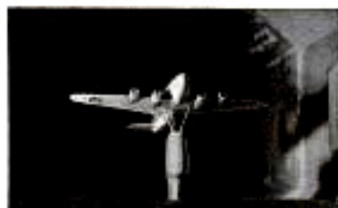
Miniature of the Stratoliner being tested in University of Washington wind tunnel
