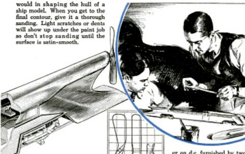
At this stage it's a good idea to give the wood a thin coat of shellac. Figs. 2 and 3 give you a clear idea of how the motor is mounted to drive the propeller. Dimensions of the mo-
