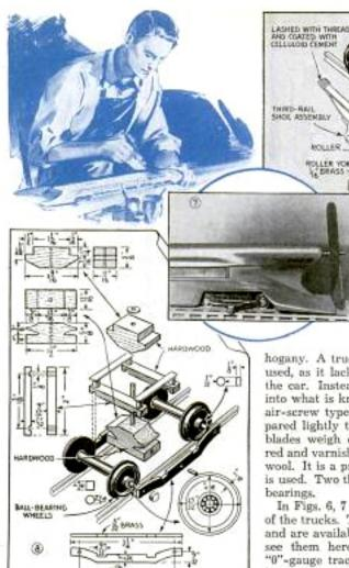
friction. Before you line it up permanently, notice that there is a sleeve bearing just ahead of the coupling. This is made "freefloating" by lashing it with heavy thread to a base, made of flat brass and screwed to the roof. With this in place you can line up the shaft. Wood putty is forced in around the bushings to hold them in place as in Fig. 2. Do the same if you use the single bushing, or log.
