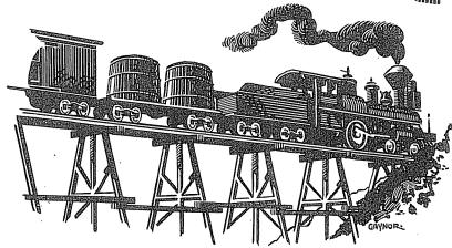
FIRST SHIPMENT OF PETROLEUM IN A TANK CAR - A FLAT CAR FITTED WITH TWO WOODEN TANKS RE-SEMBLING INVERTED TUBS-ORIGINATED AT TITUSVILLE, PA., NOVEMBER 1, 1865.
