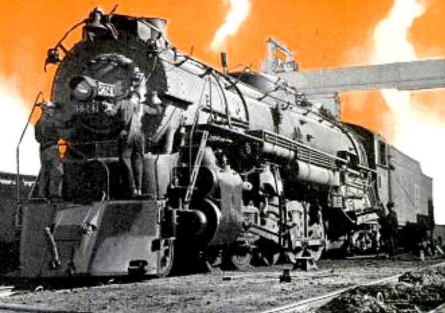
Just in from Minneapolis, No. 5624 submits to thorough inspection by electricians and mechanics in Chicago yard while fire is "pulled." Note ash buckets in adjoining track.
