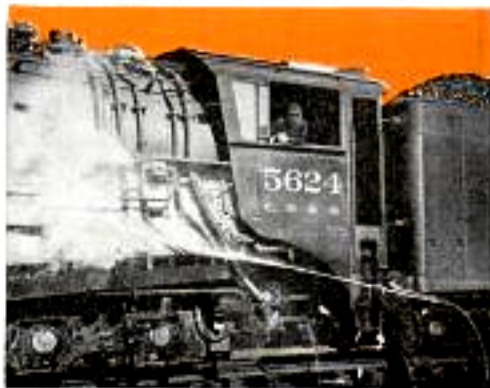
Before entering roundhouse, entire locomotive is bathed with mixture of hot water, light oil and air shot from spray gun
