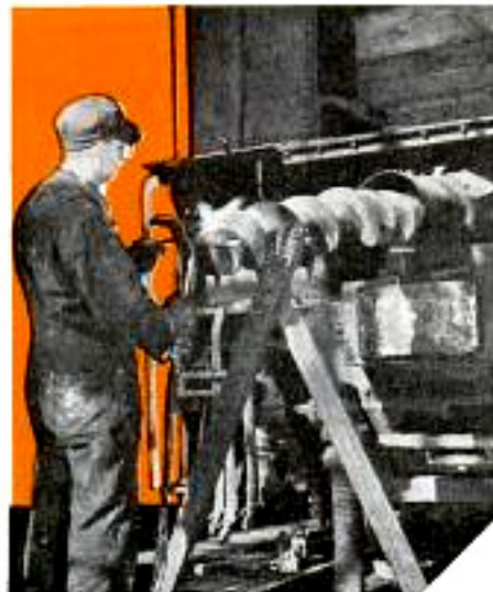
"Messy" repairs occasionally include tresh work on the stoker arena, which delivers coal from tender to locomotive firebox
