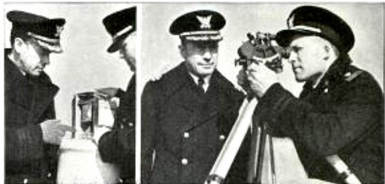
Top, left, Lieutenant Commander Edward M. Smith, commanding the cutter "Chelan," and Lieutenant Ned Strow preparing radio meteorograph for trip aloft; right, sighting departing balloon with theodolite, to compute wind velocity and direction
