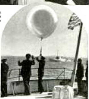
Left, attaching radio meteorograph to balloon, which must be checked for proper carrying weight. Parachute is provided to bring instruments down slowly after balloon bursts in stratosphere. Above, releasing automatic weather observer, which rises until it disappears but continues signaling
