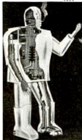
Above, showing mechanism which enables the robot to do his tricks. Center, the giant walking. Right, using the joints. The robot's brain takes consist of forty-eight electrical relays. His spinal column is made of wire—enough of it it would encircle the world at the equator
