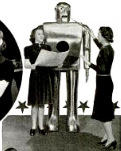
Top, left, showing some of the electrical units used to control the mechanism. Right, the robot sings through his vocal mechanism, his mouth waggling open and shut. The robot is made of 200 parts, the frame is steel and the covering is aluminum. His tricks include walking, talking, distinguishing colors, smoking and having
