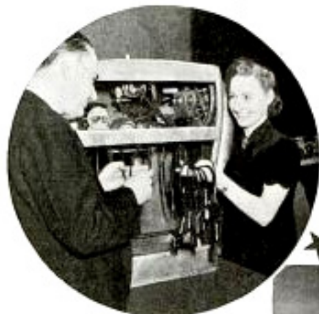
This is "Elektro," the seven-foot robot built by Westinghouse. Motors, relays and other mechanisms enable him to perform thirty-six tricks
