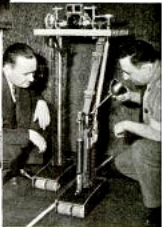
Top, left, showing some of the electrical units used to control the mechanism. Right, the robot sings through his vocal mechanism, his mouth waggling open and shut. The robot is made of 200 parts, the frame is steel and the covering is aluminum. His tricks include walking, talking, distinguishing colors, smoking and having
