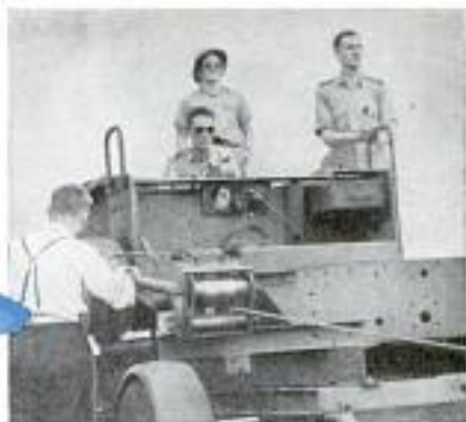
Drum of this winch revolves at constantly increasing speed to wind up towrope and launch the glider
