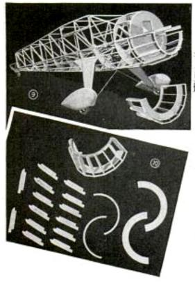
is braced in a triangular fashion to the front and rear of the longerons. The braces run from the motor mount to the landing gear at station 5 on both sides. At the rear they run between stations 6 and 7. The center piece fitted directly underneath the fuselage is held together by a rubber band, the strength of which may be increased or decreased until the proper spring action is secured. Wheel pants are carved from balsa to the size given in Figs. 5 and 8. The wheels used are 3 in. in di-
