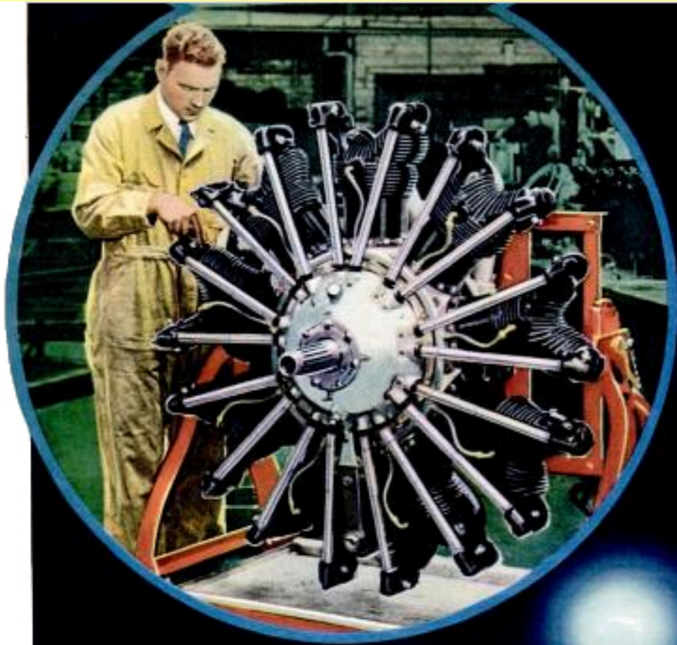
TRANSPORT plane standing in front of the Union Air Terminal, Los Angeles, before its midnight departure for the north Pacific coast cities. Left, preparing an overhauled engine for a several hours run on the test block at Cheyenne.
