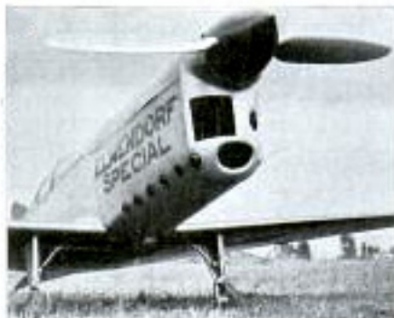
The tiny ten-inch landing wheels retract into the low wing of this racing plane
