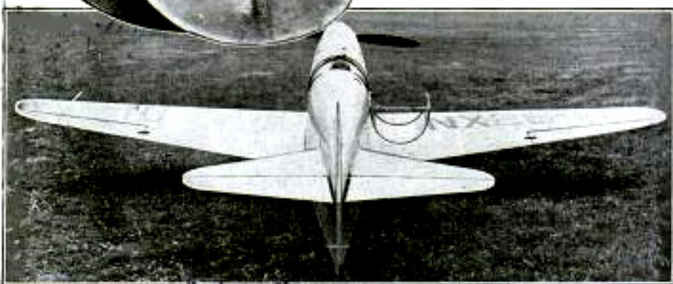
Top, working on tail assembly of new racing plane. Center, odd-shaped fuel tank fits into fuselage behind cockpit. It is designed to take advantage of every cubic inch of space. Bottom, rear view shows streamlining of racing ship. The fuselage is just wide enough to accommodate the in-line engine
