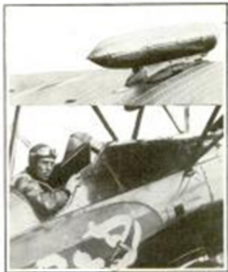
The Life Raft Is Encased in Streamlined Metal and Mounted on the Top Wing
