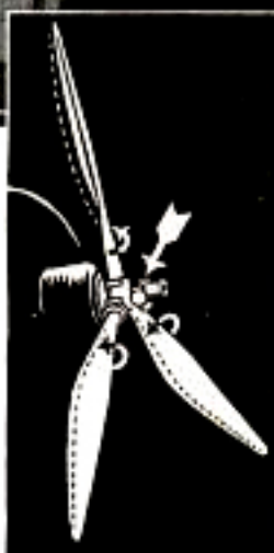
Diagram Shows Action of Controllable Pitch Propeller; Arrow Indicates Gears Which Change Pitch
