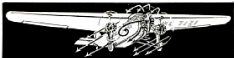
A Tri-Motor Transport with Lines Indicating Slipstream from Three Motors and Showing Why Nose Motor Is Less Efficient Than Others
