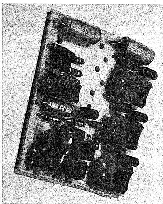
Completed Decoder board with all components in place but less the servo and battery lead wires. Note mylars folded down over other components.
