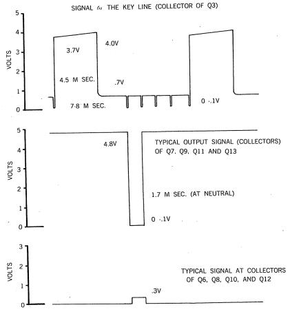
NOTE—USE 4.7K OR 10K RESISTORS IN SERIES WITH SCOPE LEADS TO PREVENT LOADING DOWN THE CIRCUIT AND CAUSING MISTRIGGERING.
