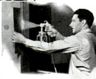
Cardboard strips can be used for a large percentage of spraying jobs where masking is necessary
