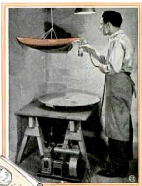
Right, work suspended on strings for finishing. Below, construction of a simple turntable
