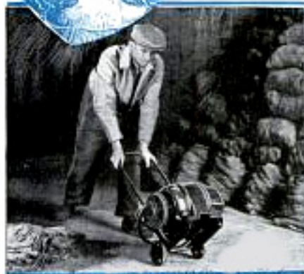
Electricity is moving to the farm. Here is a portable two-horsepower motor used to grind feed, shell corn and haul hay on a Pennsylvania poultry farm.
