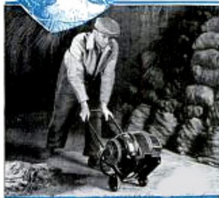
Electricity is coming to the farm. Here is a portable two-horsepower motor used to grind feed, shell corn and haul hay on a Pennsylvania poultry farm.
