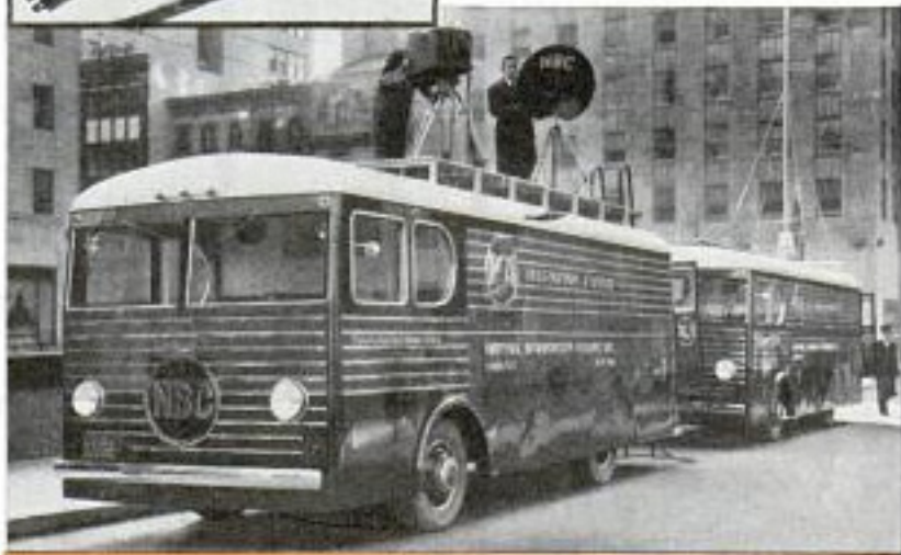
Top, watching television pictures on indirect viewing mirror under lid of receiver, which has twelve-inch kinescope and thirty-six tubes. Center, the kinescope receiving tube and iconoscope, "eye" of transmitter. Below, mobile television station which picks up image and sound in the field
