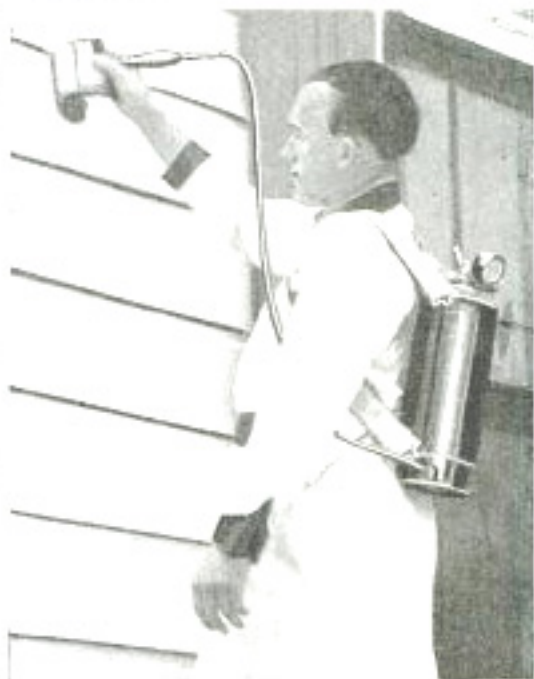
Paint is fed smoothly to bristles under control of valve in handle, eliminating dipping of brush
