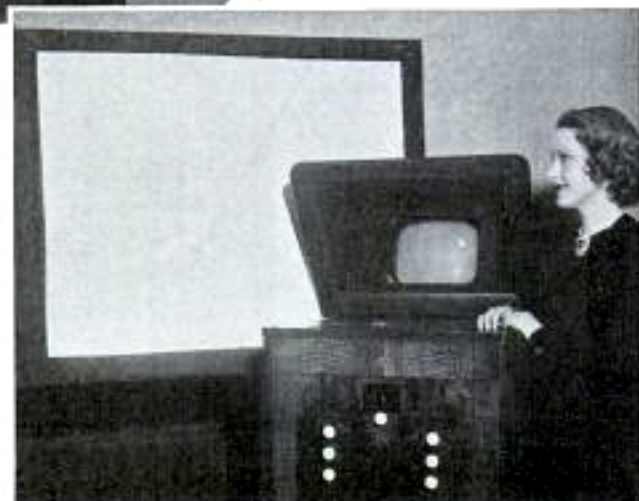
Regulation television receiver and three-by-four-foot screen on which image was "stepped up." Above, "Kinescope" projection tube which cast enlarged image on screen
