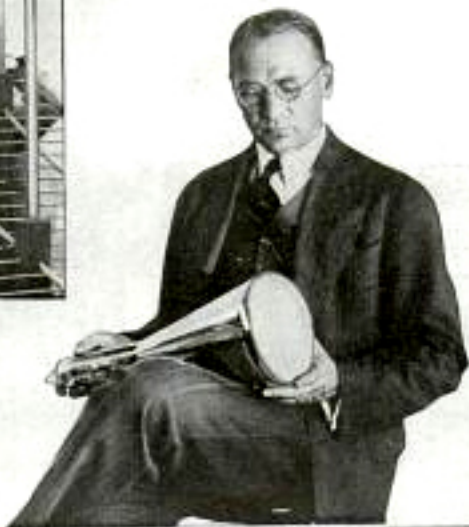
Micro-Wave Aerial System with Parabolic Reflectors; It Is Used in Experimental Work
