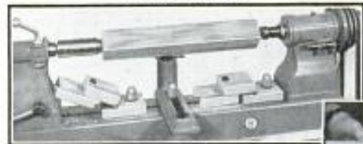
RAPID CENTERING IS MADE POSSIBLE WITH THESE SIMPLE ADJUSTABLE CENTERING BLOCKS. WHEN THE WORK IS HELD BETWEEN CENTERS THE BLOCKS ARE FOLDED DOWN TO PERMIT TURNING
