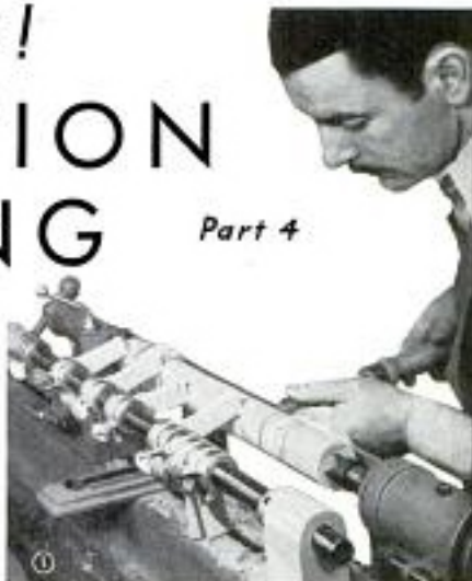
THE "SEMAPHORE" JIG IS USED TO SET OFF ALL IMPORTANT DIAMETERS AND LENGTHS OF THE TURNING
