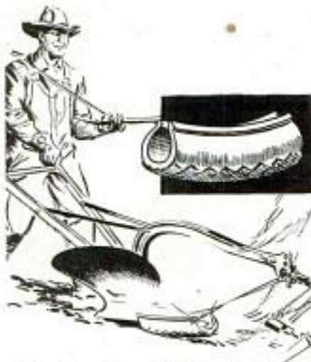
When a piece of auto tire is held under the plowshare you can move a walking plow easily
