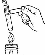
Always heat liquids carefully, not too deep into the flame and with the mouth of the test tube **pointing away** from you and everyone else in the room. Liquids sometimes spurt when heated. Also, gently shake the tube in a circular motion as you heat it.
