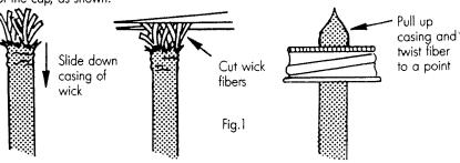
Trim the wick to a dome shape and remove all frayed and ragged strands. Keep the tip trimmed and at a height of about 1/4" for an even flame.
