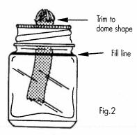
After filling the lamp, wash your hands thoroughly to remove any alcohol. Before lighting, place the lamp in a shallow metal pan filled with water.
