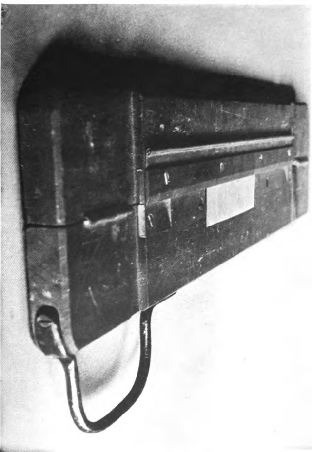
Wooden roofing folder with a piece of tin inserted ready to fold
