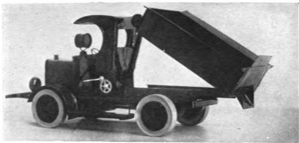
Dumping truck with body hoisted by winch under seat, made by Miss M. C. Newman
