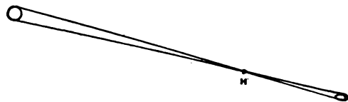
Fig. 11. The rays cross at the nail hole
