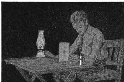
Fig. 31. Finding the candle power of the lamp
