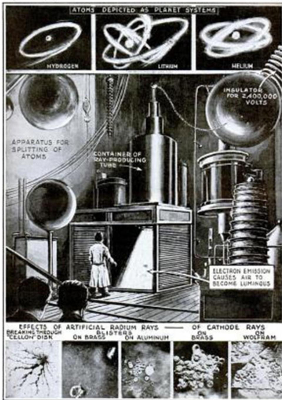
Apparatus in Center Is Used by German Scientists to Split Atoms without Employing Radium by Shoving Helium or Hydrogen Electrons at Low Voltage against Material to Be Disintegrated.
