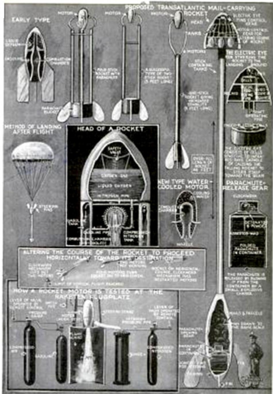
Some of the Earlier Types of Rockets That Have Been Used Successfully as Compared with the Proposed Transatlantic-Mail Rocket: Nitro Parachute-Kerosene Gas
