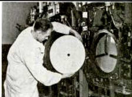
Original record goes into vacuum-sealed chamber of top to be coated with gold. Bottom, placing record in machine where it is coated with copper.
